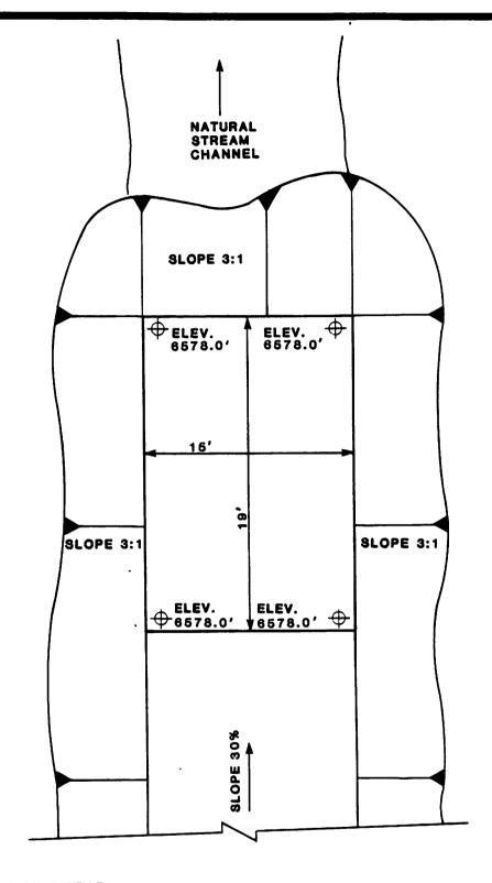
MINIMUM HEIGHT OF RIPRAP ALONG SIDEWALLS ABOVE THE BASIN FLOOR = 5.3'
