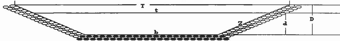
**Riprap - Steep Slope Design - PADER Method**
