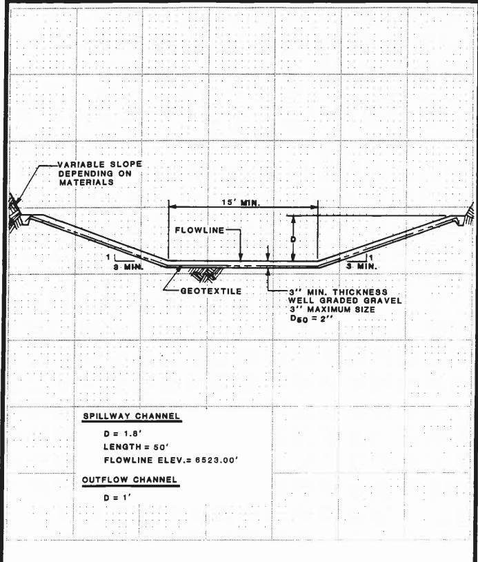
SPILLWAY AND OUTFLOW CHANNEL CROSS SECTION N1-M
