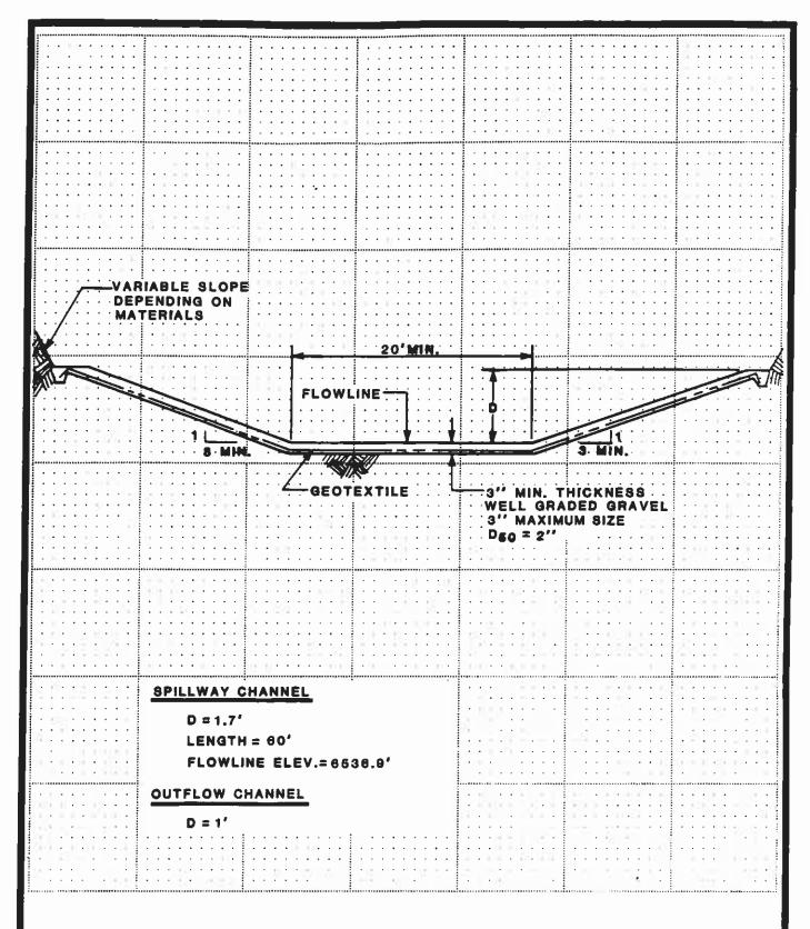
SPILLWAY AND OUTFLOW CHANNEL CROSS SECTION J7-CD
