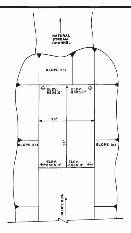
MINIMUM HEIGHT OF RIPRAP ALONG SIDEWALLS ABOVE THE BASIN FLOOR = 3.2'
