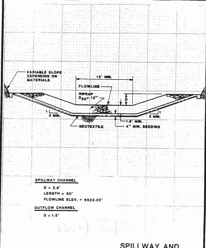
SPILLWAY AND OUTFLOW CHANNEL CROSS SECTION J3-B
